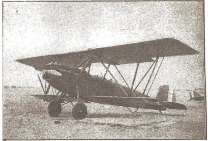
Here's a real prize for you collectors. Many years ago, the Air Corps used this Huff-Daland for observation work. An American-built Hiss supplied the power. Note heavy interplane bracing.
