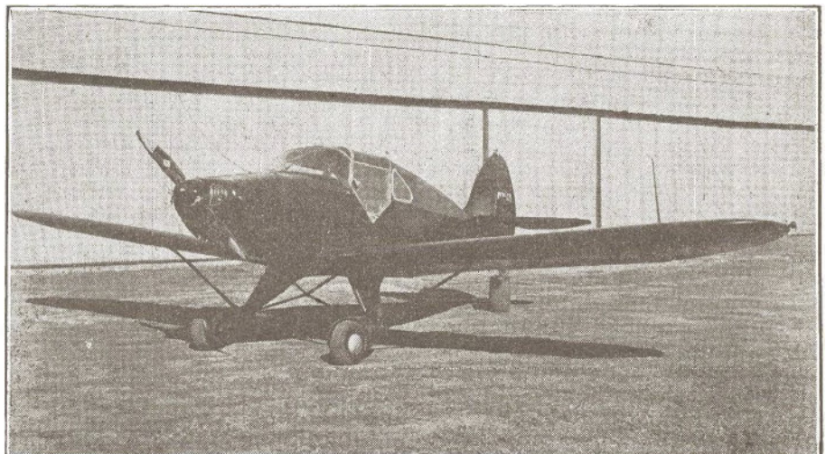
This new Ariel light job can be had with three different engines—Lycoming, Continental, or Franklin. Top speeds, in order: 115, 125, 127.
